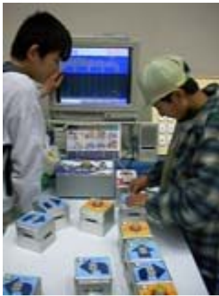
Figure 1: Various examples of tangible user interface. Top: the interface doll ActiMates Barney that can function as a playmate for children [1]. Bottom: the new learning tool called ArgoBlock which enables the students to learn how to construct computer programs without knowing any programming language [3].
