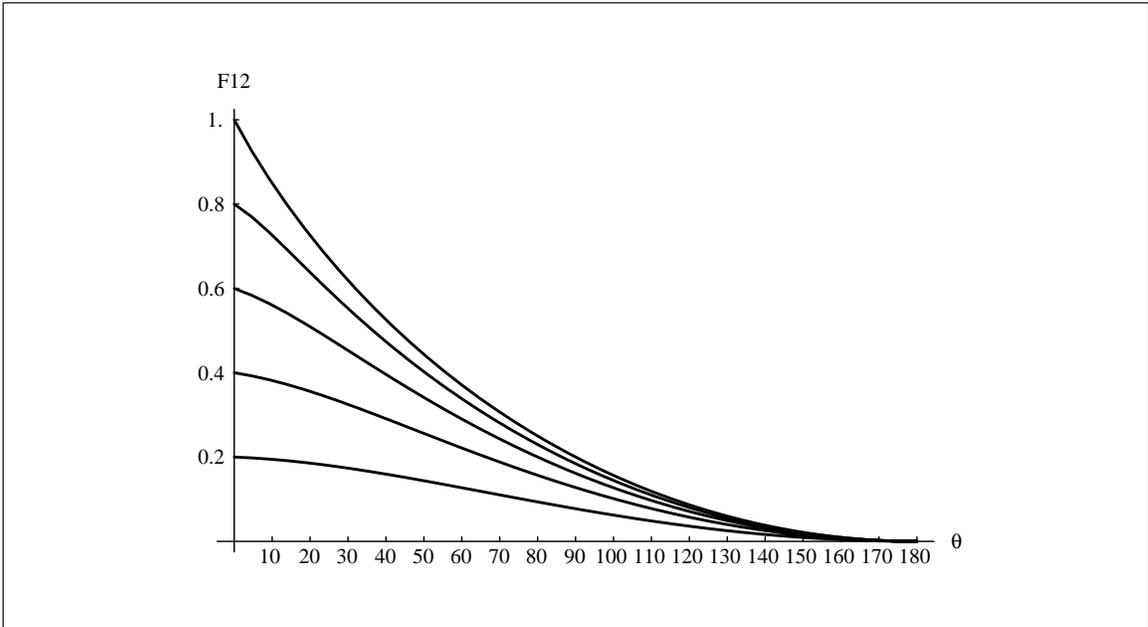
Figure 4: The form factor for the geometry in Figure 3 as a function of  $\theta$  for edge ratios  $l = \frac{a}{b}$  of .2, .4, .6, .8, and 1.0.
