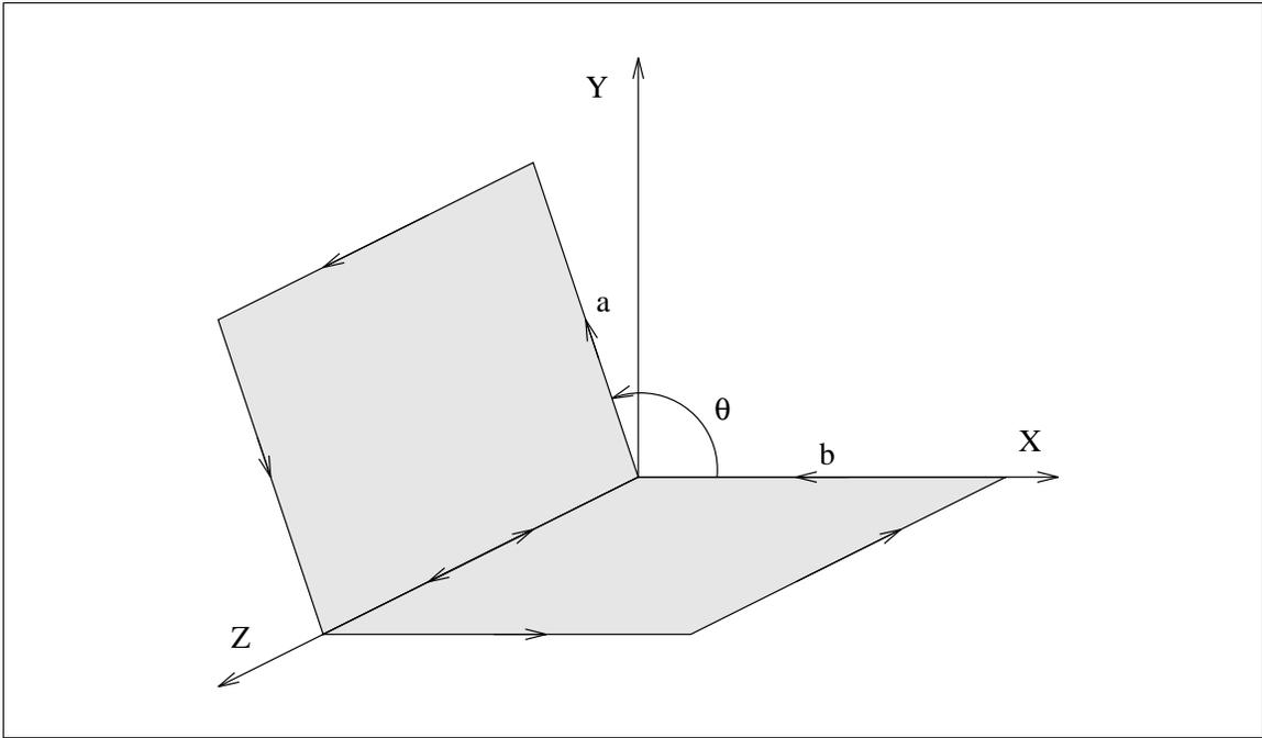
Figure 3: Geometry for two rectangles sharing a common edge with an enclosing angle of  $\theta$ .
