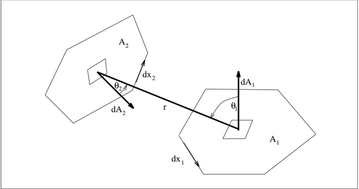
Figure 1: Geometry for the form factor between two surfaces  $A_1$  and  $A_2$ . The differential surface elements are shown as  $d\vec{A}_1$  and  $d\vec{A}_2$ , making the angles  $\theta_1$  and  $\theta_2$  respectively with the connecting vector  $\vec{r}$ . The boundary elements are shown as  $d\vec{x}_1$  and  $d\vec{x}_2$ .
