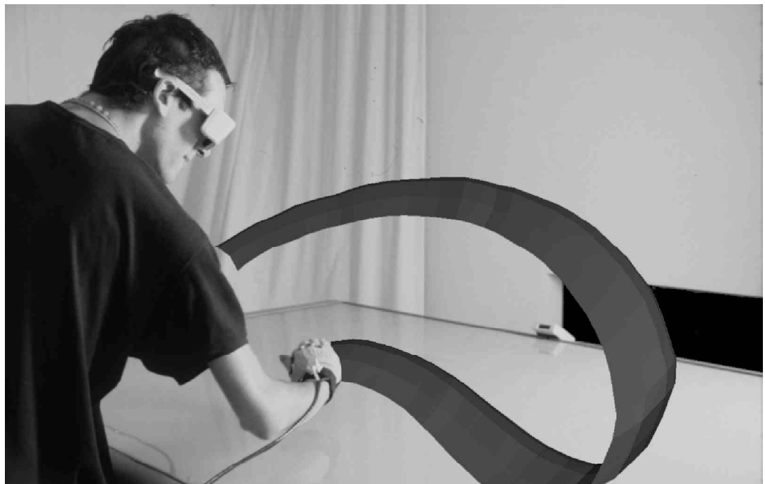
Fig 1. A thin strip of surface is drawn with the hand. Special viewing hardware makes the stroke appear to float above the table, as depicted in this composite image.
